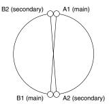
If a problem occurs with the main heads, for example if only one channel is being recorded and playback cannot be done, you can temporarily switch to the secondary heads so that the playback picture can be viewed.
